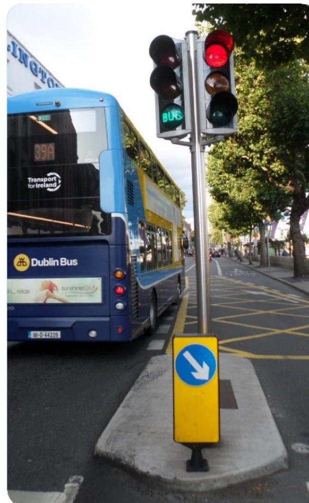
Figure 2: Signal Controlled Bus Priority
