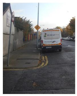
The presence of traffic signs along this section of the route was minimal, however it was noted at the junction between Pembroke Cottages [northbound] and Cambridge Road that some poles were located directly in the line of travel. These traffic signs shall be relocated out of the direct line of travel as part of the overall design and construction of the scheme.
