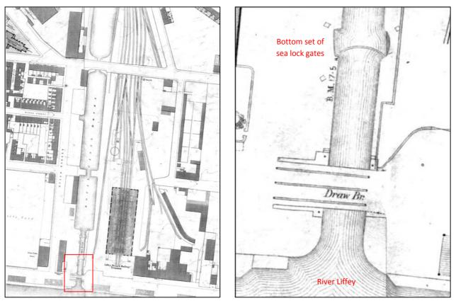
Fig 3.3 1864 map showing the Royal Canal Dock and new moveable bridge at its entrance from the Liffey. The bridge moved west when being opened (OS 1:1056 map, Dublin City sheets 15 and 16).
