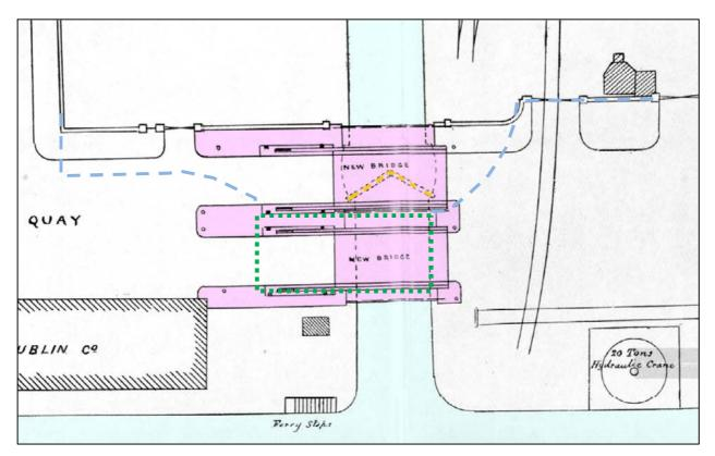
Fig 3.7 John Griffith's Scherzer bridges. The outline of the replaced rolling drawbridge is shown in green. The previous wall along the north side of the road (shown as a dashed blue line) was moved back to accommodate the new inner bridge, under which was the bottom pair of sea lock gates (*Griffith 1912, fig.5*).
