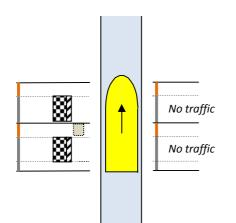
**3.** Inner Bridge now raised to let boat pass under. Outer Bridge remains raised so both bridges are now closed to all road traffic.
