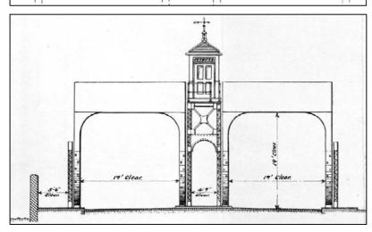
Fig 3.8 Scale drawings of the Scherzer bridges (*Griffith 1912, figs 6-8*).
