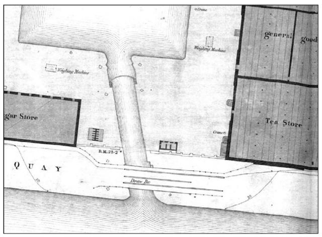
Fig 6.4 1864 map showing the new rolling drawbridge at the entrance to George's Dock The entire bridge moved eastwards when being opened (OS 1:1056 map, Dublin City sheet 15).
