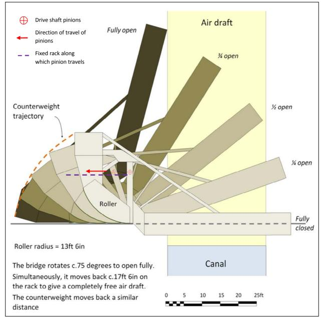
Fig 1.3 Operation of Scherzer bridge (based on Royal Canal, Dublin).
