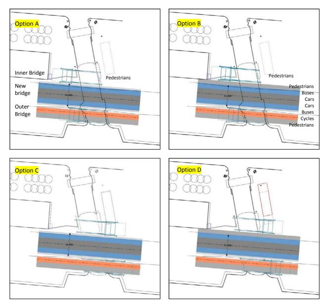
Fig 8.2 Options for repositioning Scherzer bridges.
