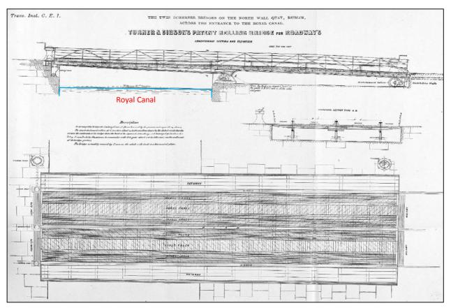
Fig 3.2 Elevation (looking south) and plan of drawbridge across canal entrance (Griffith 1912, fig.2).
