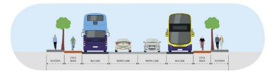
Figure 4-1: Typical CBC Cross Section
